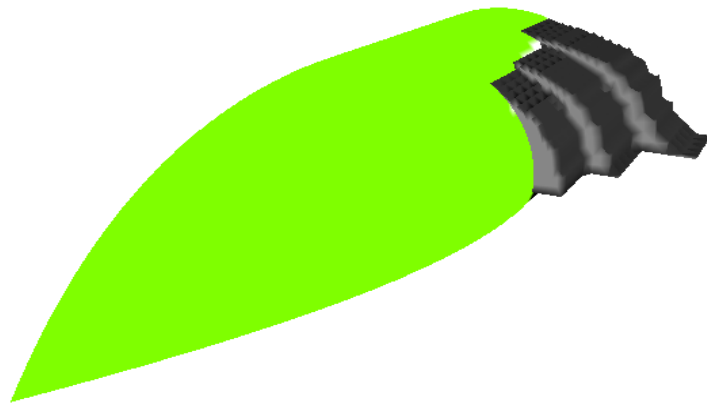
Figure 4.39: Finned Missile: The iso-surface of separation layer.
